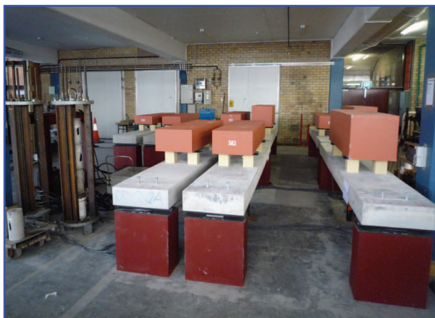
Figure 1: Slab specimens under sustained loads
