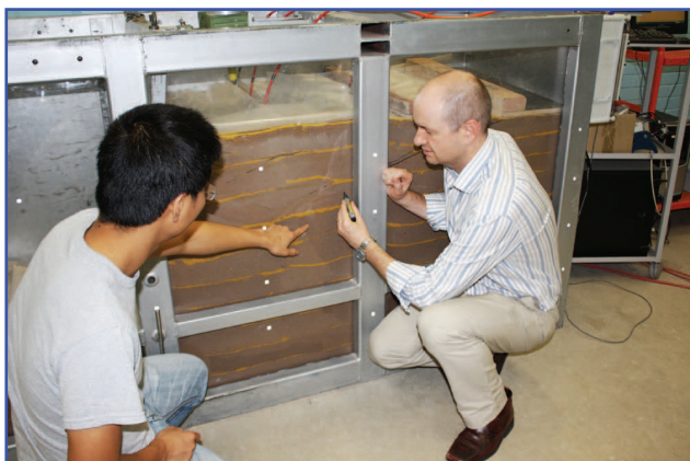
Dr Adrian Russell (right) and Mr Liem Vo (PhD student) observe the laboratory controlled failure of an unsaturated soil adjacent to a retaining wall.
