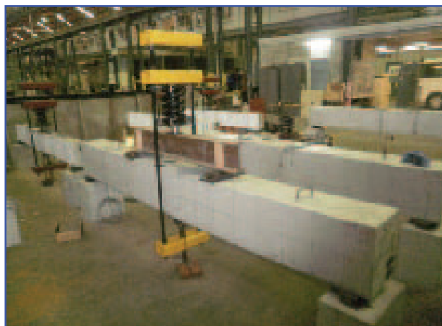
Figure 2: Beam specimens under sustained loads
