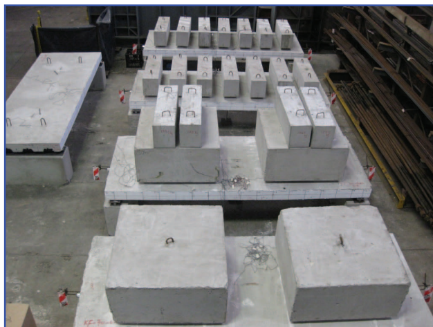
Slabs under sustained loads
