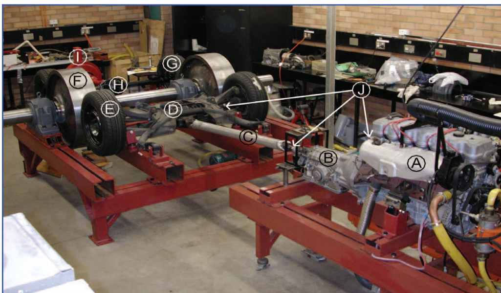
UTS vehicle test rig Components A Engine B Automatic Transmission C Propeller D Fwd final drive E Fwd tyres F Flywheels (four more to be added) G Rear tyres H Rear final drive I Dynamometer J Torque sensors
