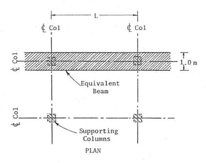
Figure 2 The 'Equivalent Beam' in a Flat Slab or Flat Plate.
