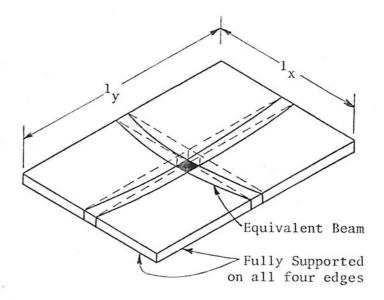
$\frac{\text{Figure 1}}{\text{Edge Supported Slab}} \quad \text{The 'Equivalent Beam' in a Two-Way}$
